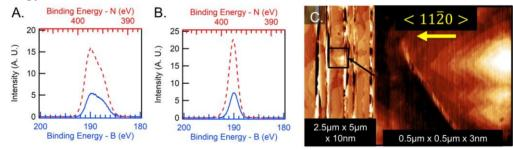
Fig. 1: XPS spectra of the B 1s (solid blue) and N 1s (dashed red) core levels from CBE growth (A) and plasma-assisted CBE growth (B) using borazine at 1450°C on epitaxial graphene substrates. The lack of lower binding-energy peaks in Fig. 1B indicate phase-pure films. Fig. 1C shows atomic force micrographs of h-BN on epitaxial graphene after a 1450°C growth, with a closeup of a multilayer h-BN domain. The underlying SiC substrate <11-20> direction is indicated.
