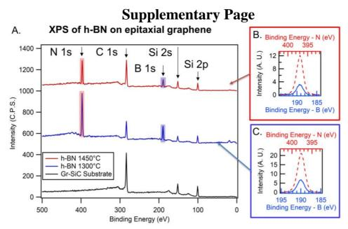
Fig. S1: A) X-ray photoemission spectra showing survey scans of the as-loaded epitaxial graphene on 4H-SiC(0001) substrate (black) and the CBE deposited BN films at 1300°C (blue) and 1450°C (red). The insets show the B1s and N1s core level peaks, corresponding to a ratio of 84% B:N (nitrogen rich) for the 1300°C deposition and 70% B:N for the 1450°C deposition as referenced to a CVD-grown control. According to XPS substrate peak attenuation, the film is approximately 9Å or ~3 monolayers thick.
