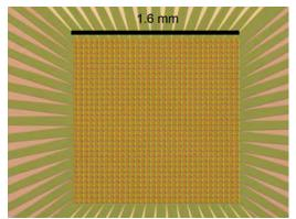
Figure 1 : Optical micrograph of a 32 x 32 array of SNSPD detectors
