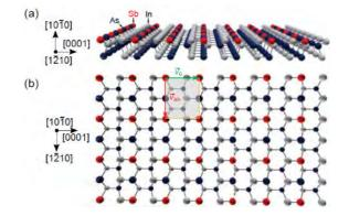
Figure 1 Perspective view of a ball model of the two-dimensional idealized (long range) chemical ordering of the monolayer shell on the InAs sidewall facet, based on the ordering and antiordering vectors extracted from pair correlation function. (a) Side and (b) top view with surface unit cell.
