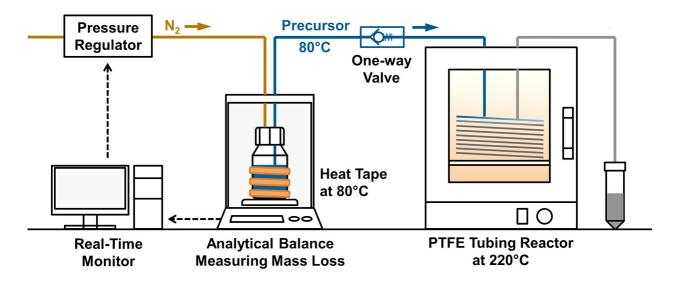
Figure 1. Representative continuous flow nanofabrication device
