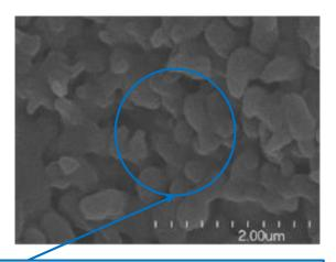
The snail shells have 200 nm porous structures, and an oil repellent function in water.
