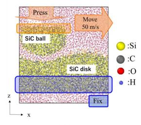
Fig.1: Simulation model of sliding interface of SiC in water.
