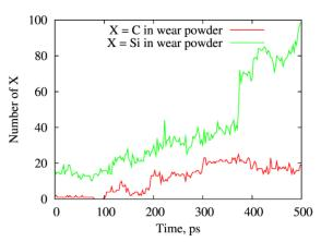
Fig.4: Change in the number of Si and C contained in the wear debris .
